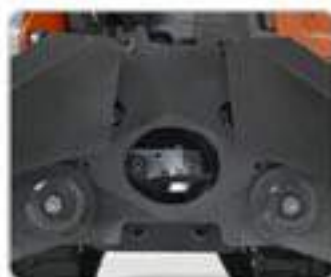
Convenient handle for track release.
