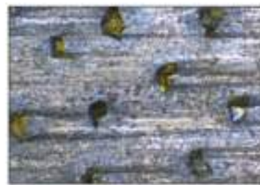
Based on the Diagrip2™ technology which distributes the diamonds at equal distance in a 3-dimensional matrix inside the segment, Diagrip2™ additionally optimizes the distribution of the active surface.
