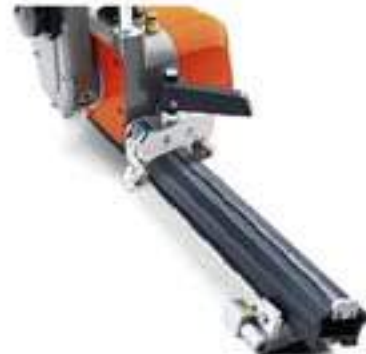
Quick mounting of sawhead on rail.
