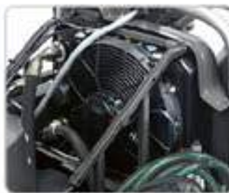
Electric fan for extra efficient cooling.
