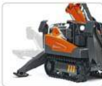
Individual control of the outriggers.
