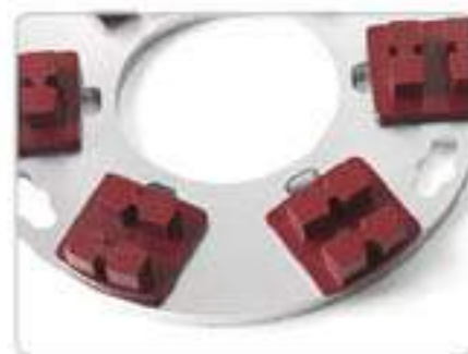
Low-profile disc holder with recessed locking mechanism reduces overall height of tooling, increasing the efficiency of dust extraction.
