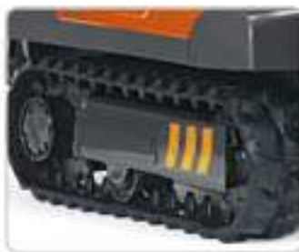
Hydraulic track tensioning as standard.
