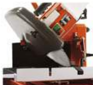
Tiltable head for angle cutting.
